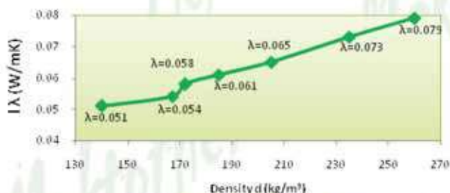
Thermal Conductivity dependance on mortar density
